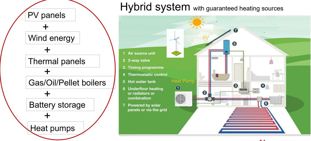
Due to the request of decarbonization, HP+PV should be the main stream for future application
