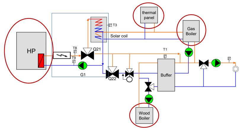
Hydraulic Connection for heating/cooling and DHW charging with buffer tank including wood boiler/gas boiler/thermal solar support for heating and DHW
