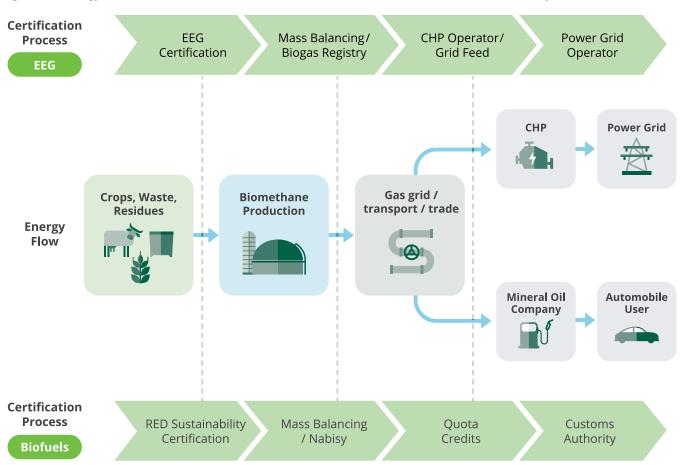
Figure 17: Energy flow and certification/cash flow for the biomethane certification and incentive system.
