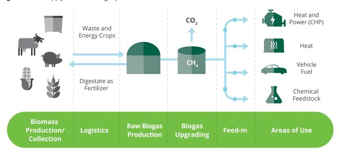
Figure 1: Value supply chain for a biogas plant.
